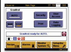
Process Control's Gravitrol Gravimetric Extrusion Control Systems automate the control of any extrusion line – monoextrusion or coextrusion – on the basis of weight. The EXB2 Operator Station is the key component of a complete Gravitrol system.
